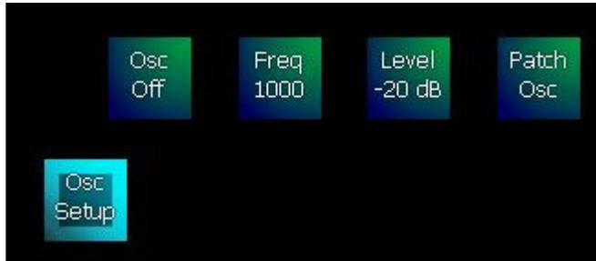
The Frequency and Level buttons will cause the Numpad to display when pressed. You can type in the required number, then press Frequency or Level again to accept the new value and exit.
